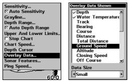
Overlay Data command on the Sonar Menu (left). Overlay Data Shown selection menu (right). In this example, we scrolled down the data list to highlight Ground Speed.
